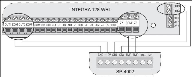
Fig. 20. Connection of siren with own power supply (by the example of SP-4002) to control panel outputs. The OUT2 high-current output is programmed as the supply one. Audible signaling is triggered by OUT3 output, and optical signaling by OUT4 output (low-current outputs with normal polarization: when activated, they are shorted to ground). Z8 is programmed as tamper zone (NC type, function 9. 24H TAMPER).
