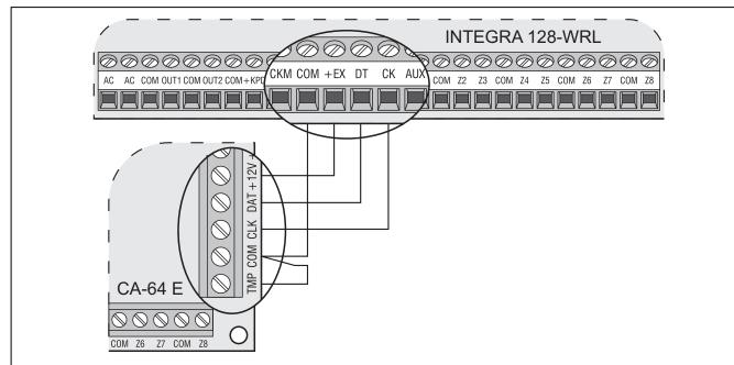
Fig. 10. Connection of modules without power supply unit, by the example of CA-64 E zone expander. The expander is mounted in the same housing as the control panel, hence the TMP terminal is shorted to the COM ground.
