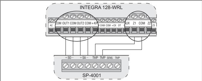
Fig. 19. Connection of siren without own power supply to high-current outputs (by the example of SP-4001). Optical signaling is triggered by OUT1 output, and audible signaling by OUT2 output (high-current outputs with normal polarization: when activated, +12 V voltage is supplied). Z1 is programmed as tamper zone (NC type, function 9. 24H TAMPER).
