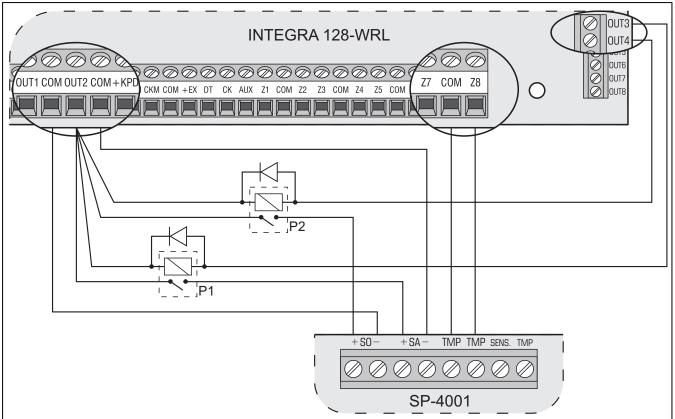
Fig. 21. Connection of siren without own power supply (by the example of SP-4001) to control panel outputs. The OUT2 high-current output is programmed as the supply one. OUT3 output controls P1 relay which triggers audible signaling. OUT4 output controls P2 relay which triggers optical signaling. Z8 zone is programmed as tamper zone (NC type, function 9. 24H TAMPER).
