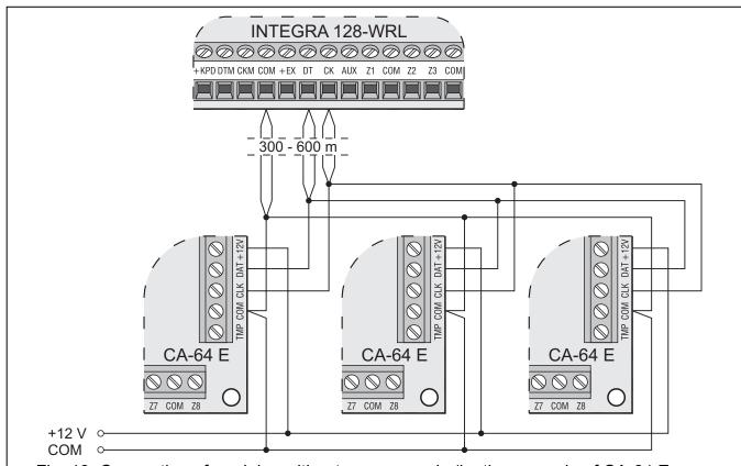
Fig. 13. Connection of modules without power supply (by the example of CA-64 E zone expander) to the control panel – the distance between panel and modules is 300 to 600 m. The modules are powered from a control panel independent source (power supply/expander with power supply). 2 wires in cable are used for each signal (CK, DT, COM).
