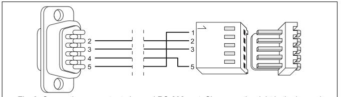
Fig. 9. Connecting computer to keypad RS-232 port. Shown on the right is the keypad interface. Shown on the left is the DB-9 female connector from soldering points side.
