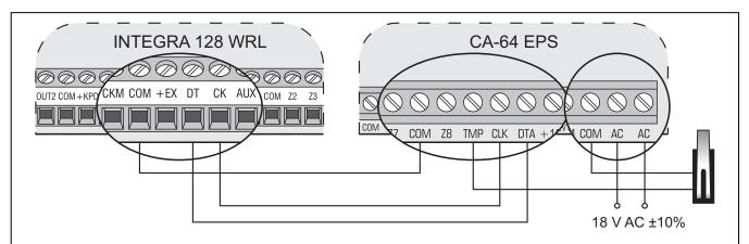
Fig. 11. Connection of expansion module with power supply unit, by the example of CA-64 EPS zone expander. Housing tamper contact is connected to TMP and COM terminals. AC terminals should be connected to transformer secondary winding terminals.
