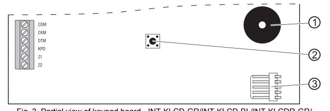
Fig. 3. Partial view of keypad board - INT-KLCD-GR/INT-KLCD-BL/INT-KLCDR-GR/INT-KLCDR-BL.
