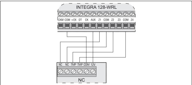
Fig. 14. Exemplary connection of NC type detector to control panel (NO type detector should be connected in the same way).
