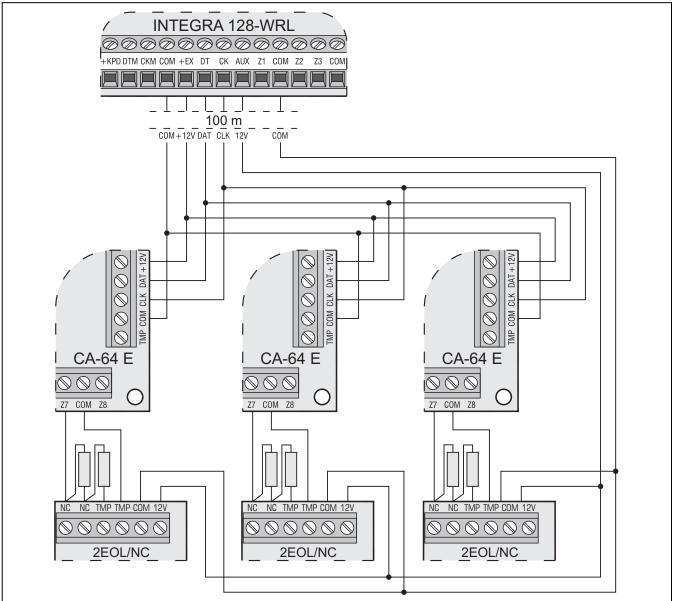
Fig. 12. Connection of modules without power supply to the control panel when the distance between panel and modules is small (by the example of CA-64 E zone expander). Several modules (connected in parallel) are connected to the control panel lead-in. Expanders only may be connected to the +EX power terminal. Detectors must be supplied by separate power leads.
